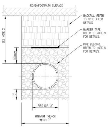
TRENCH BACKFILL AND BEDDING (STD - W - 13) SCALE 1:20
