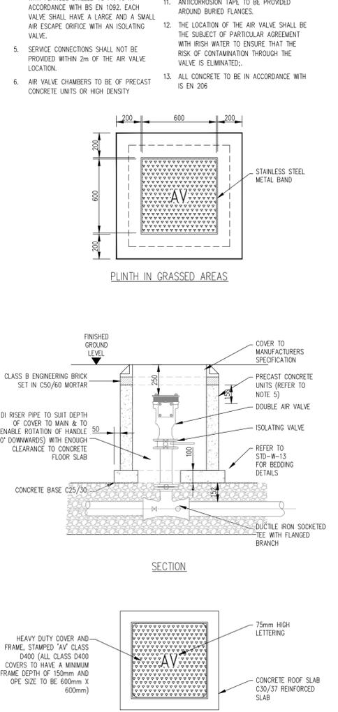
AIR VALVE CHAMBER (PRECAST CONCRETE CONSTRUCTION) (STD - W - 20) SCALE 1:20
